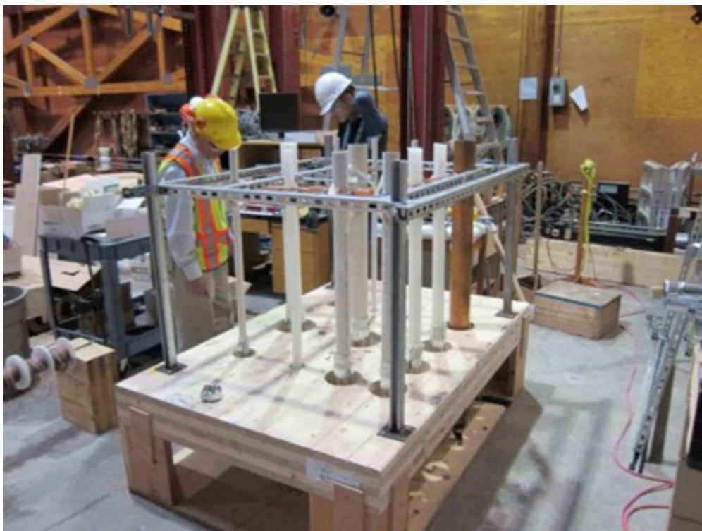
Fire testing of CLT through penetration firestopping
