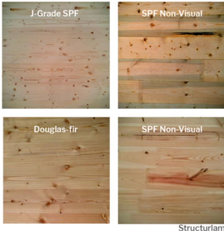
For mass timber, specification of appearance varies by product. Aesthetic expectations for cross-laminated timber (CLT) and nail-laminated timber (NLT) are agreed upon between the building designer and manufacturer/fabricator and described in the product specifications, whereas for glued-laminated timber (glulam) are standardized. Historically, appearance classifications have also been referred to as “appearance grades.” However,
