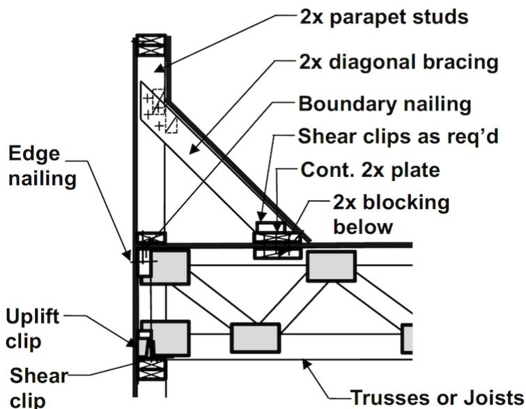
IBC Section 705.11 defines the requirements for parapets. As a default, the code requires that parapets be installed on all exterior walls of a building. However, there are several exceptions to this, notably when one of the following conditions exists:
